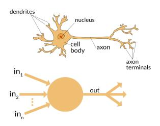
The structure of a neural network is based on biological neurons. Source: Applied Go (2016, June 9). Perceptrons - the most basic form of a neural network. Retrieved December 11, 2019 from https://appliedgo.net/perceptron/.
